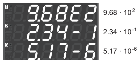
Fig. 6: Exponential illustration of the measurement channel measured value (examples)
